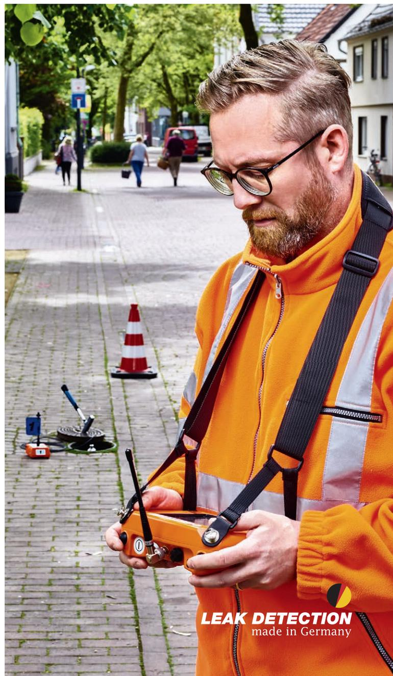
The **SeCorrPhon AC 200** is a multifunctional leak detector offering three functions in one: prelocation, pinpointing and correlation. The clever combination of these processes in one system allows you to confidently locate the leak regardless of the ambient conditions. With just a few finger strokes, you can quickly and easily switch between the various applications.
