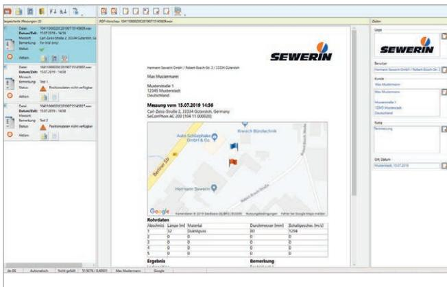
Noises which have been recorded can be played back using the player integrated into **WaterCom**. If the software is used regularly to save measurements, it will start to build up a useful noise database. This can then be used, for example, to train new starters in leak detection in what to listen out for.
