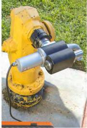
**FERROPHON® FG 155 C** Generator – All Material Pipe and Cable Locator
