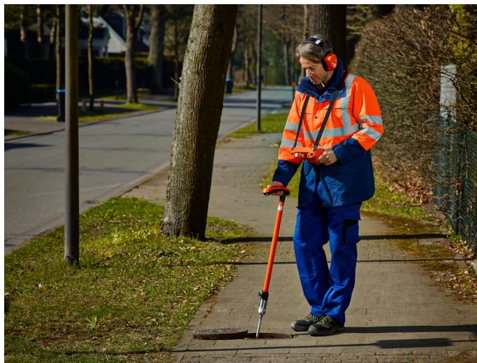
When it comes to detecting leaks in water pipes by electro-acoustic means, the hearing and experience of the user are paramount. The **AQUAPHON®** system supports and simplifies this detection process thanks to the outstanding quality of its microphone and measuring technology, intelligent analysis functions and the practical, visual representation of results on the display.
