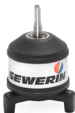
The **BM 230** ground microphone lends itself more to use on unpaved surfaces. Its solid tripod always guarantees a firm base. If the ground is particularly soft, it is possible to screw on a spike to improve the sound transmission even further.
