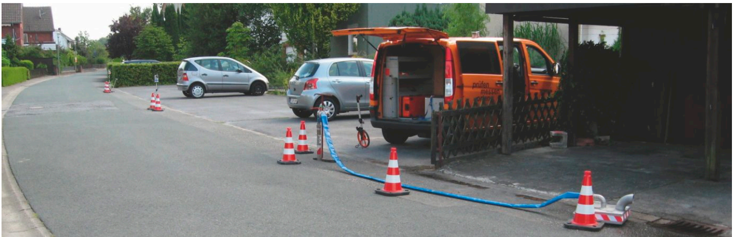
Figure 6: Setup for sound velocity measurement
