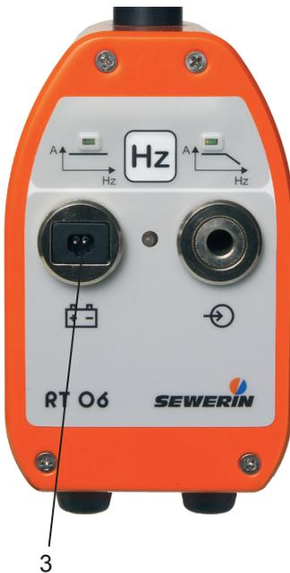
Built-in NiMH cells are used for supplying the **SeCorr 08** and **RT 06**.
