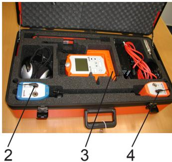
Inside the transport case, connect cables 2 and 4 to the two **RT 06** transmitters and cable 3 to the docking station HS 1,2 A.
