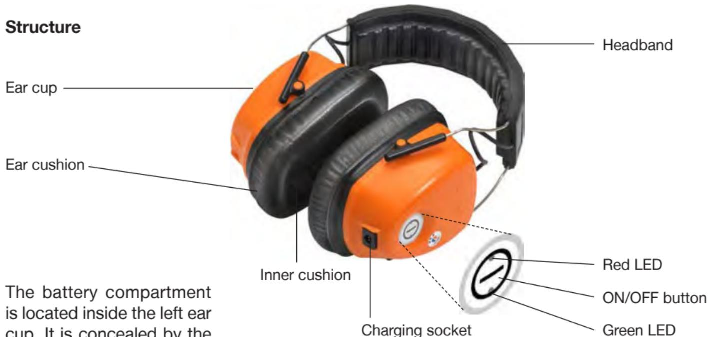
The battery compartment is located inside the left ear cup. It is concealed by the inner cushion.
