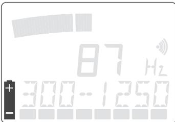
The battery symbol appears about 15 minutes before the battery runs out. In case the accumulator volume drops further, the instrument automatically switches off to protect the accumulator.
