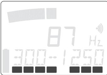
The volume display indicates the volume set. If the bar on the extreme left is shown in reverse video, the volume is low; if the bar on the extreme right is shown in reverse video, the volume is maximum.
