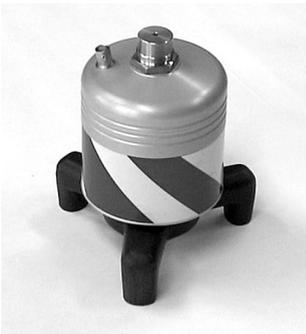
The ground microphone 3P-4 is used to locate leaks beneath unstabilised surfaces. An earth spike can be screwed onto it for use in soft ground. Its 3 feet guarantee stability at all times.
