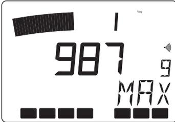
If you hold down the micro key for 3 seconds, you can switch to „MAX“mode. This mode helps with acoustic line detection. Instead of minimum values, only max values are shown in this mode (only with microphones with cable connection, not with radio microphones).
