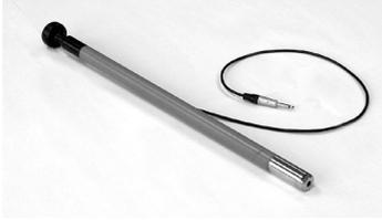
The test rod is used for preliminary leak location. The test rod is placed in contact with valves on the line under investigation.
