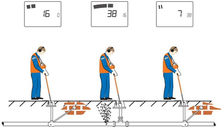
In water leak detection the display will be similar to that shown in the illustration above.
