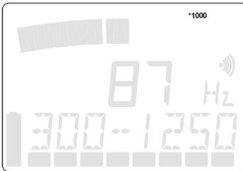
Basic amplification is useful for adapting to extreme situations. The higher the basic amplification, the louder the noise in the headphones. The values 10, 100 or 1000 appear in the display.
