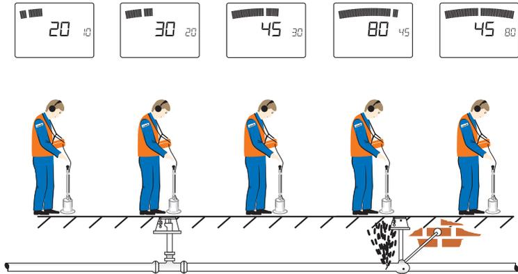
Non-metallic pipe materials do not transmit structure-borne sound as well. Therefore checking at the valves is not enough. The sections between valves must also be checked with a ground microphone.
