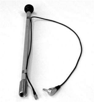
The carrying rod can be used with both ground microphones. The BO-4 or 3P-4 microphone is screwed onto its lower end.
