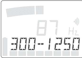
Different leak noises can be heard best in different frequency ranges, and two people may hear the same noise differently. To optimise acoustic perception a bandpass can be set. In this case only a particular frequency range is fed to the headphones. The best setting can be found by experiment, or alternatively the **A 100** can search for it automatically.
