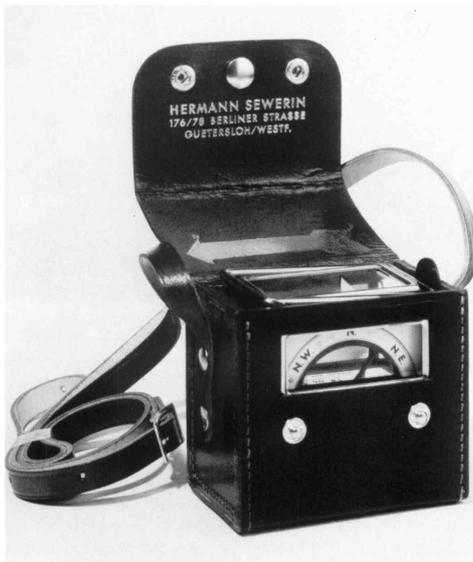
To retain the durability and performance of this instrument fully, it is recommended to use it with the case which will also prevent the instrument from receiving scratches and other damage. The instrument should not be stored near ferrow-magnetic objects (like steel shelving). This could cause the magnetizing of the needle to diminish.
