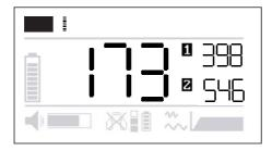
Fig. 4: Graphical and numerical noise level display in maximum noise level function
