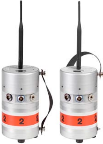
Fig. 6: Carrying handle attached to RT 300 lengthways (left) or crossways (right)
