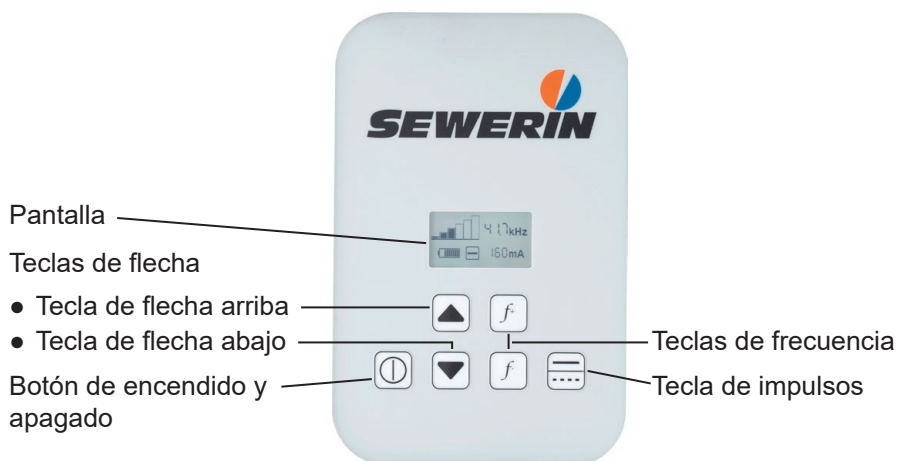
Fig. 3: Panel de control
