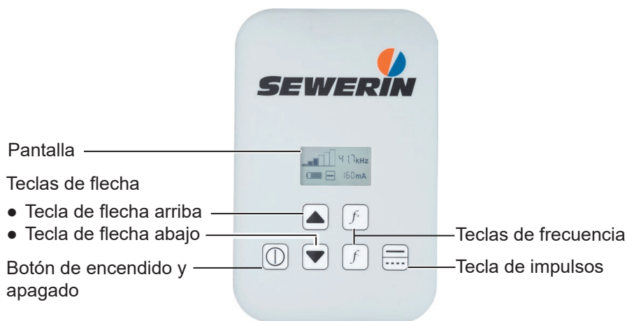
Fig. 3: Panel de control
