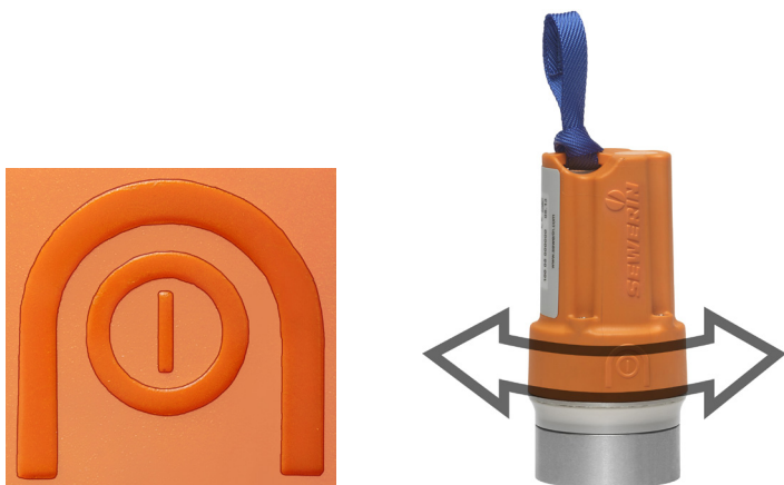
Fig. 3: Activating the Logger: Relief of activation switch on housing (left) Direction of movement of magnet (right)
