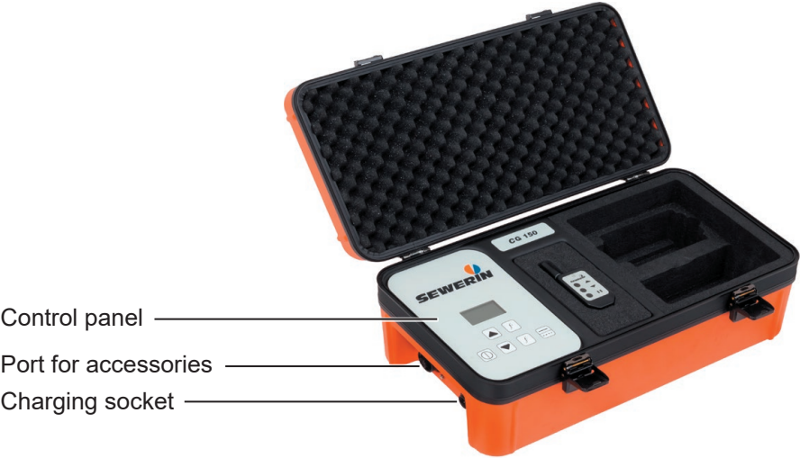
Fig. 1: CG 150 generator with an opened case
