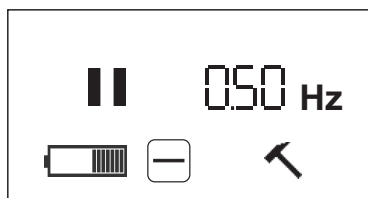
Fig. 5: Display when using the remote control ( Pause symbol)
