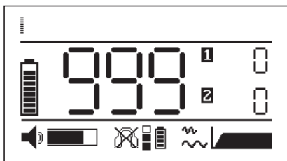
Fig. 6: System with F8 wireless headphones ready for use (battery symbol for wireless headphones visible)
