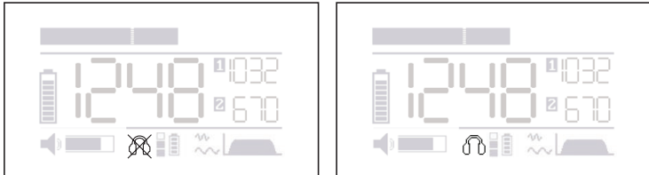
Fig. 9: Headphones symbol when the system is ready for use Image left: Symbol crossed out, i.e. no measurement in progress or hearing protection threshold exceeded during a measurement Image right: Symbol not crossed out, i.e. measurement in progress and noises can be heard
