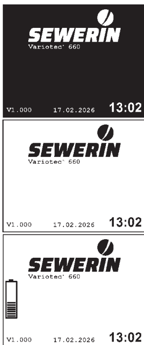
Fig. 11: Sequence of start images during switch-on process
