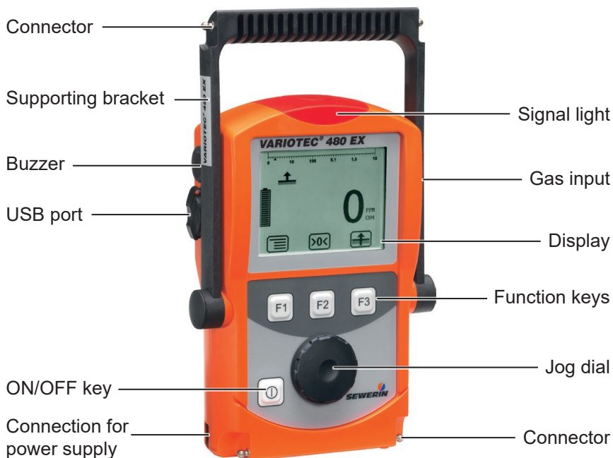
Fig. 1: VARIOTEC 480 EX device overview
