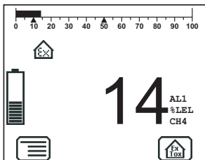
Fig. 16: Warning %LEL measuring mode
