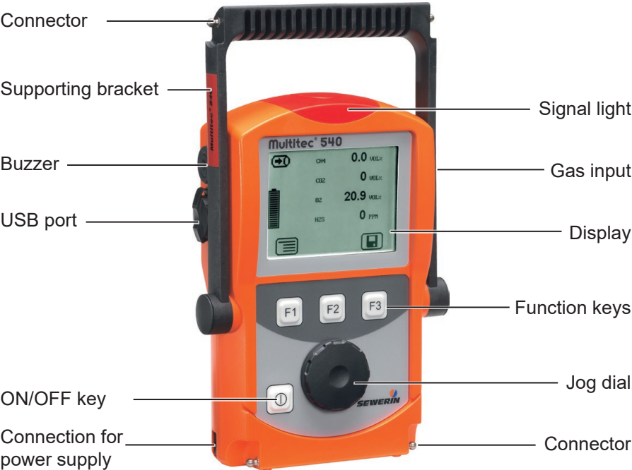
Fig. 1: Multitec 540 device overview
