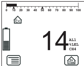
Fig. 16: Warning %LEL measuring mode
