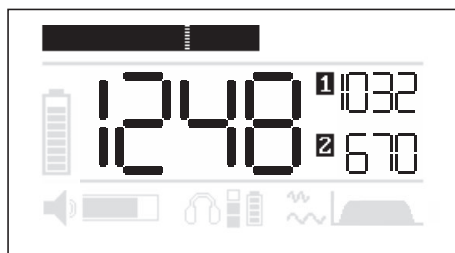
Fig. 5: Graphical and numerical noise level display for water leak detection
