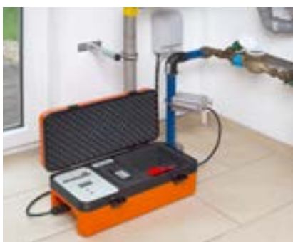
Locating metallic pipes and plastic pipes
