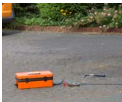
Acoustic location of main pipes
