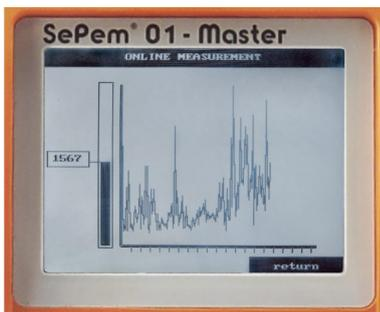
Online measurement, as illustrated here, allows you to determine prior to installation if a "zero measurement" might even be possible during the day.
